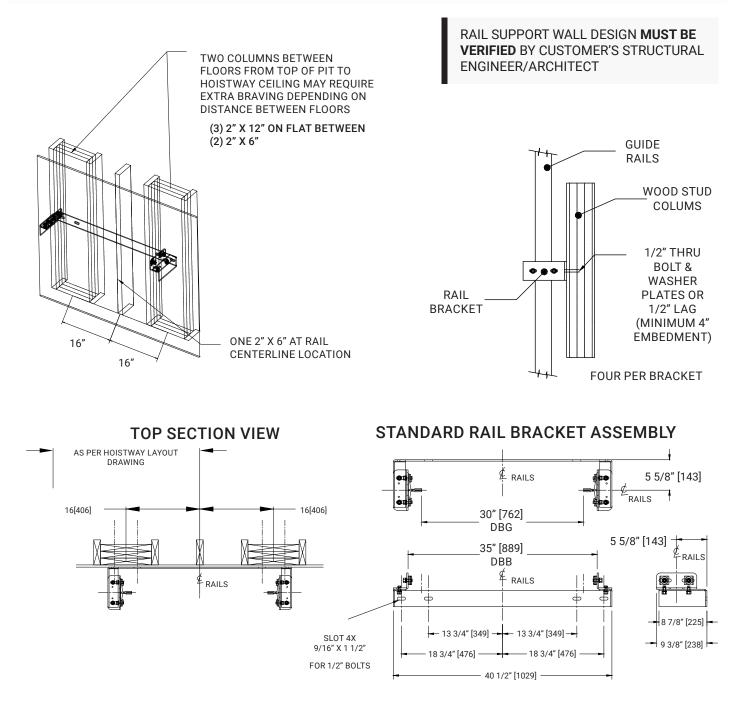
THE ELEVATOR DEVICES CODE REQUIRES THAT THE BUILDING CONSTRUCTION FORMING THE SUPPORTS FOR THE GUIDE RAIL BRACKETS SHALL BE DESIGNED TO WITHSTAND THE FORCES AS INDICATED IN THE DRAWING PACKAGE. THE GENERAL CONTRACTOR SHALL ENSURE THAT THE APPROPRIATE PROFESSIONAL (ARCHITECT AND/OR ENGINEER) REVIEW THE INDICATED FORCES TO ENSURE THAT THE BUILDING DESIGN/CONSTRUCTION MEETS ALL REQUIRED CODES.
